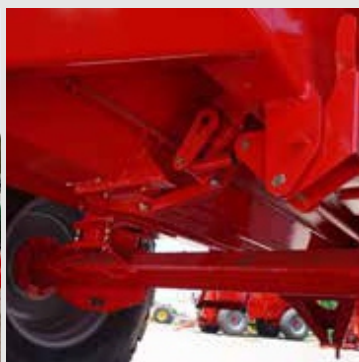
Sliding bottom doors.
