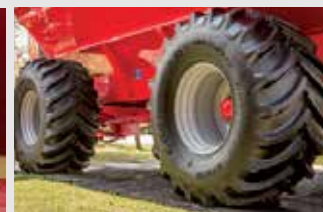
High flotation tires with minimum soil compaction.
