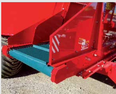
Hydraulically operated right-side discharge PVC belt conveyor.
