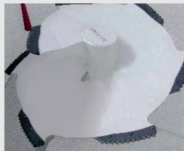
Auger with tungsten carbide coated knives.
