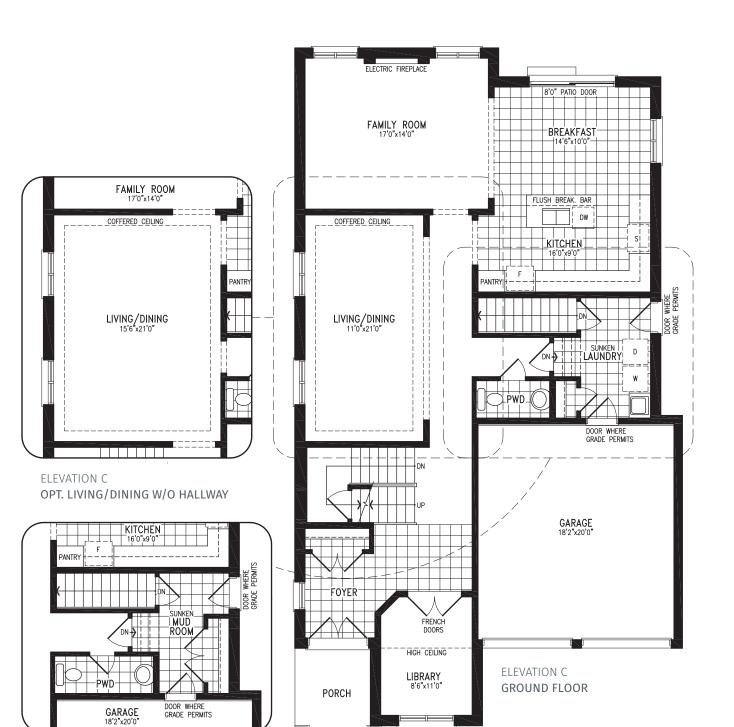
ELEVATION C OPT. MUD ROOM (Laundry to Basement or Second Floor)
