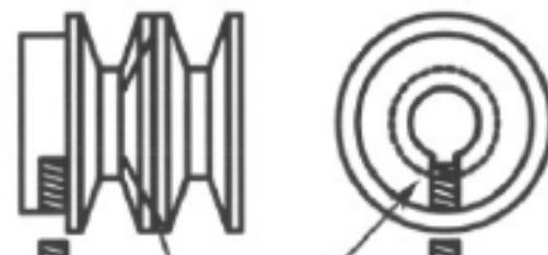
0126 6" diameter pulley. 2 Groove for gas Honda engine.
