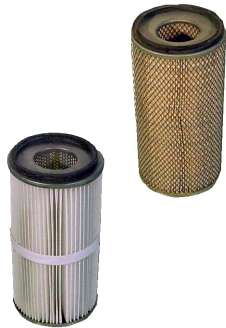
2505797 (Standard) Spun Bond Poly w/ PTFE Coating 99.995% Efficiency @ .03 Microns
