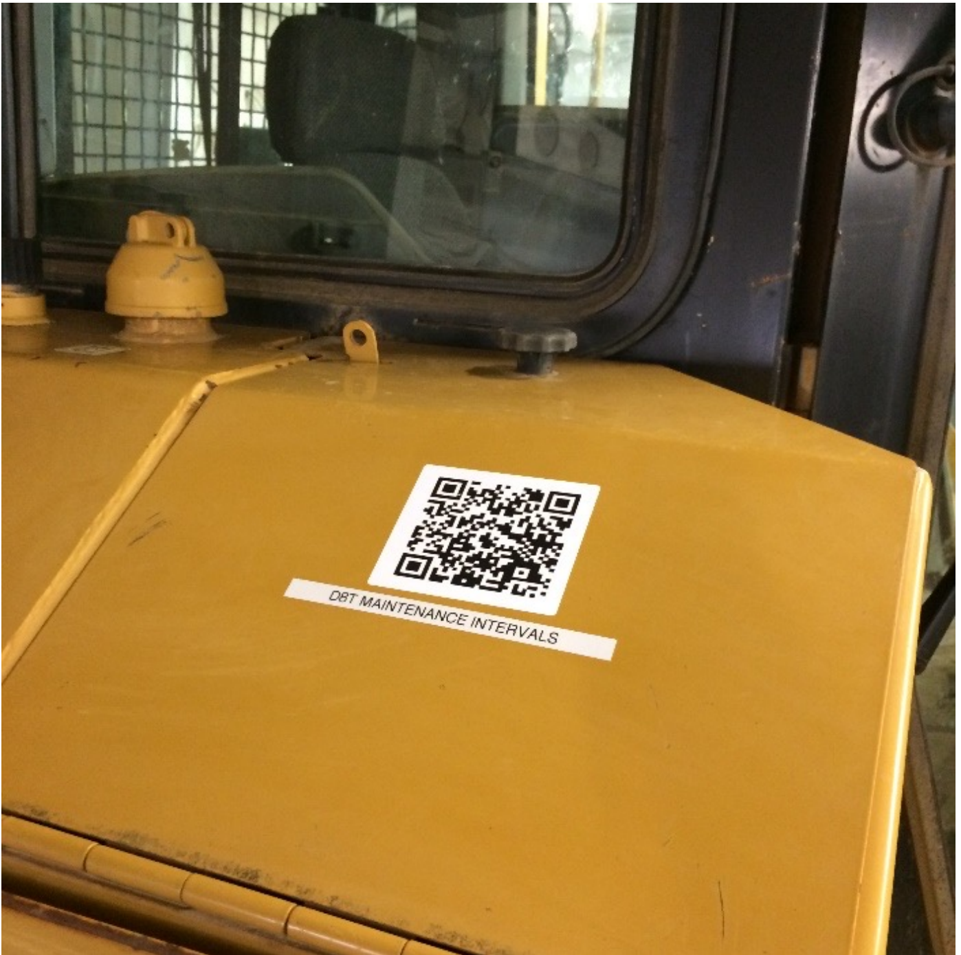
The QR codes throughout Henkels & McCoy's fleet provide instant smartphone access of key construction equipment information to service technicians and operators, including a dozer's maintenance intervals. // Source: Gil Gilbert
