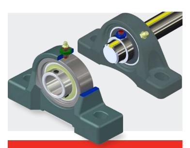
AMI offers two types of custom locking devices that are both designed to accommodate axial shaft expansion caused by high temperatures from an oven application. The two design options are specifically intended for the expansion side of an application. (Float side). \*A fixed mounted ball bearing unit should be used on the opposite side of the shaft.\* (Fixed and Float setup).
