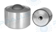
Hardened machined steel housing without flange, internal thread on the bottom for fixing with screws or threaded bars, turned steel cover, felt seal\*. Available in steel, zinc plated steel, stainless steel. Balls in chrome steel, 420 stainless steel, plastic material.
