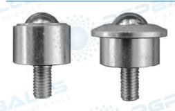
Hardened machined steel housing, threaded nut machined from solid\*, cover in turned steel, no felt seal to ensure better smoothness. Available in steel, zinc plated steel, stainless steel. Balls in chrome steel, 420 stainless steel, plastic material.
