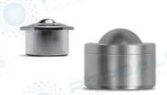
High-performance machined, case-hardened and hardened steel housing. Removable turned steel cover\*, felt seal, drain hole on the bottom. Available in steel, zinc plated steel, stainless steel. Balls in chrome steel and stainless steel AISI 420.
