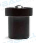
External housing in turned, burnished steel. Internal unit all made of machined, hardened and zinc plated steel. Felt seal. Internal spiral spring. Available in burnished steel, stainless steel. Balls in chrome steel, AISI420 stainless steel. Fully removable.
