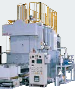
Vacuum carburizing of transmission gears.
