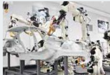
Spot Welding System
