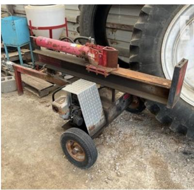
MTD log splitter features a 20-ton cylinder and is powered by an Intek I/C 206 Briggs & Stratton engine. It's equipped with 4.80/4.00-8 tires and is a solid, dependable splitter.
