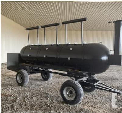
1,000-gal Smoker – Heavy-duty pit with 41" doors, temperature gauges, and solid steel construction. Fire box is 46" wide, 51" long, and 30½" tall, with a 36" door with adjustable vents and an ash tray for easy cleanout. Gear is on 11L-15 tires. A great setup for large-scale smoking.
