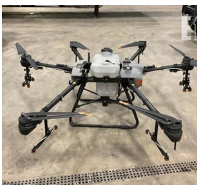
DJI Agras T30 agricultural spray drone in excellent condition. 6-inch front/back and 12.5-inch left/right wing nozzle spacing, 8-gallon tank with quick-fill cap, and includes a T30 Spreader System 3.0 (never used).
