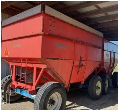
Killbros 375 wagon in solid condition. 12-ton running gear, adjustable hitch, 11R-22.5 front tires, and 10.00-20 rear tires, ready for use.
