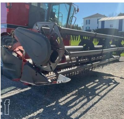
Case IH 1020 Header in good shape, 17ft cutting width, hand-crank reel slides, hydraulic reel raise/lower and height-control. Field ready
