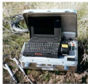
Thermal probe and property analyzer to determine the soil resistivity
