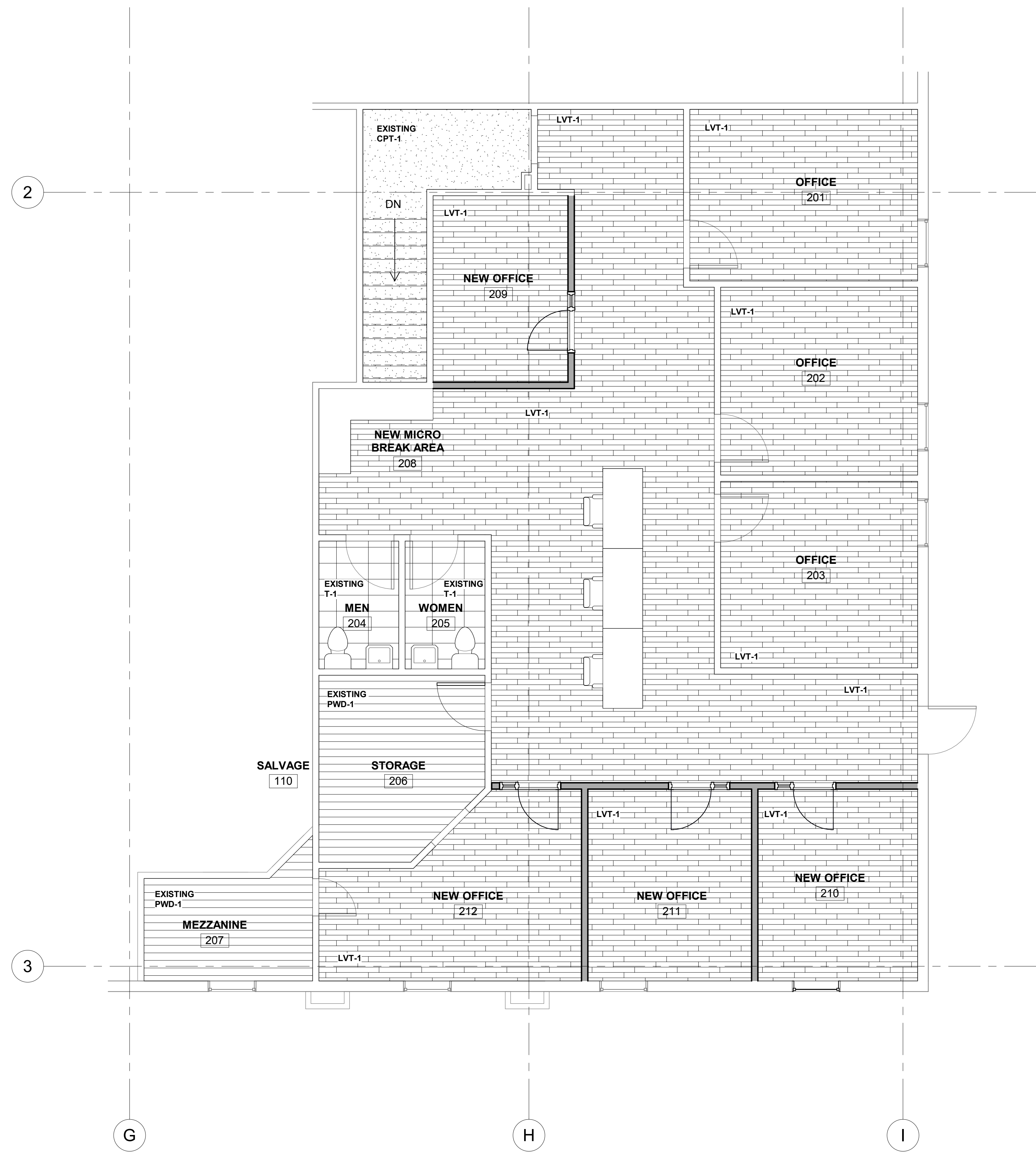
1 ENLARGED SECOND LEVEL FINISH PLAN - ADMIN OFFICES 1/4" = 1'-0"
