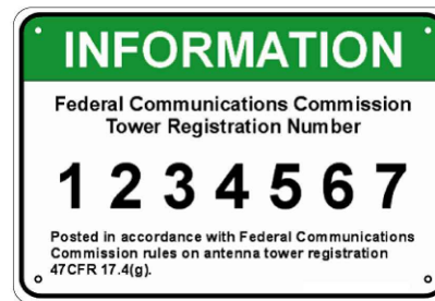
FCC REGISTRATION SIGN WHITE/GREEN BACKGROUND, WHITE/BLACK LETTERING. MOUNTING LOCATION: GATE & BASE OF TOWER. QUANTITY: 2
