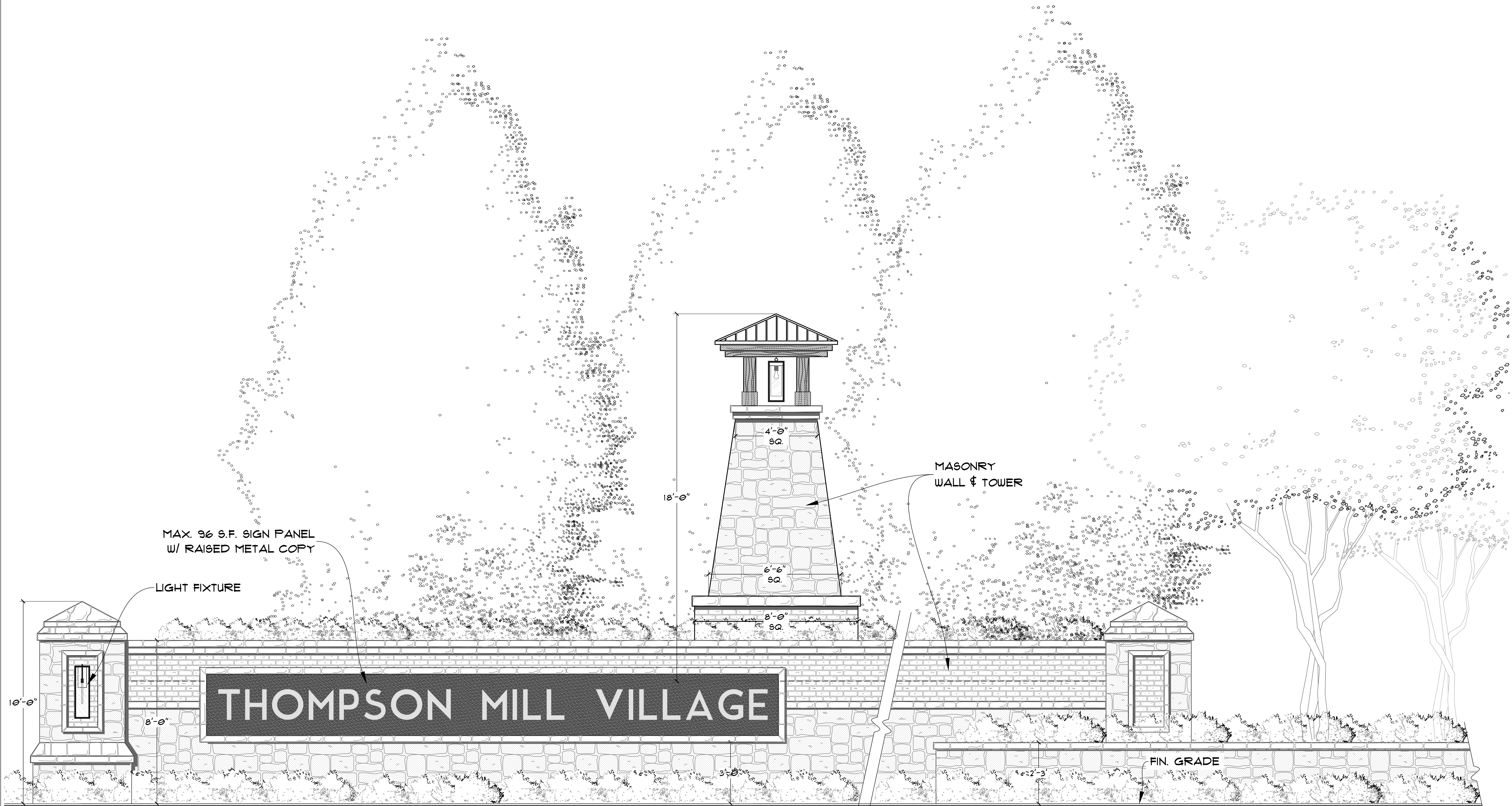
VIEW 'A' SIGN WALL ELEVATION 1/2"=1'-0"
