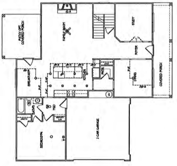
1 Main Level Electrical NOT TO SCALE
