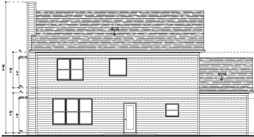
2 Rear Elevation w/ 3rd Car Garage Option A22 SCALE: 1/4" = 1'-0"
