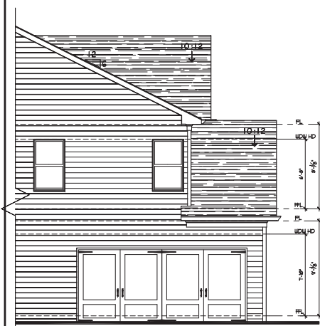
4 Left Side Elevation 'B' A12 SCALE: 1/4" = 1'-0"
