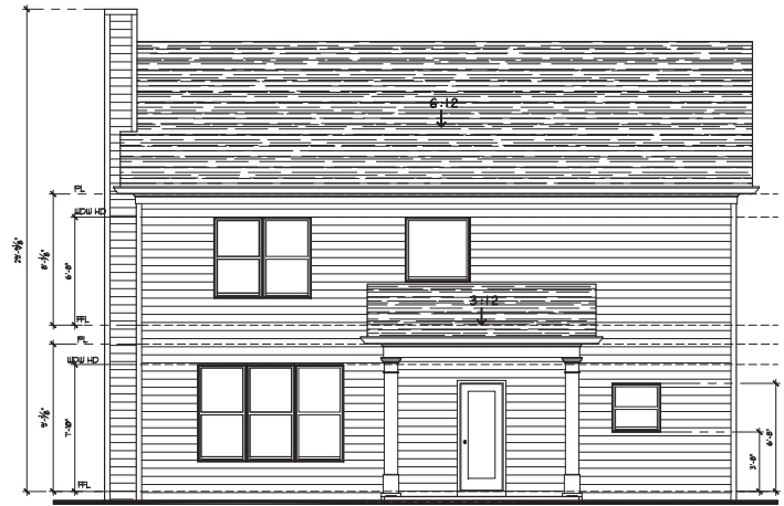
4 Rear Elevation w/ Opt. Covered Porch A2.2 SCALE: 1/4" = 1'-0" 0 4' 8'
