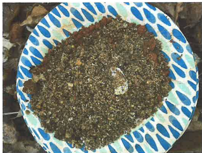
View of refusal material (weathered rock) at GGG Boring S-5.
