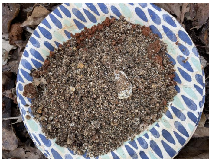
View of refusal material (weathered rock) at GGS Boring S-5.
