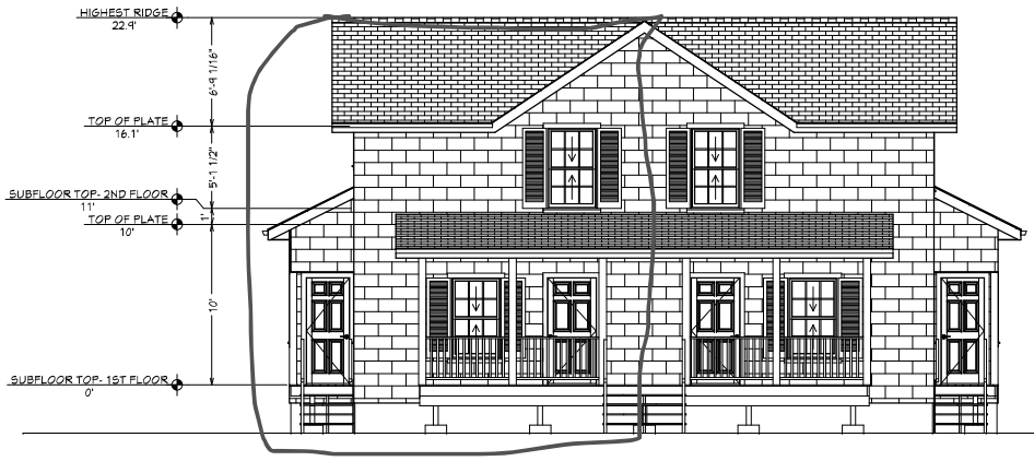
E1 Exterior Elevation Front-As-Built 1/4 in = 1 ft
