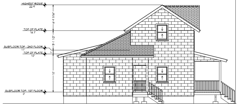
E2 Exterior Elevation Left-As-Built 1/4 in = 1 ft
