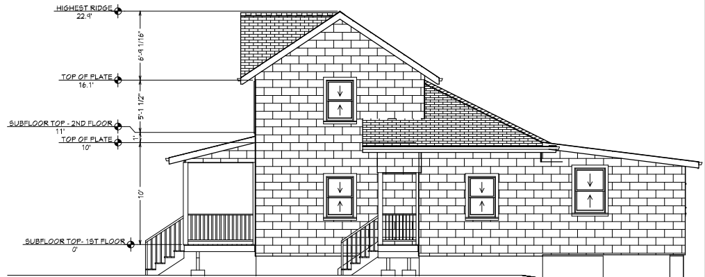
E4 Exterior Elevation Right 1/4 in = 1 ft
