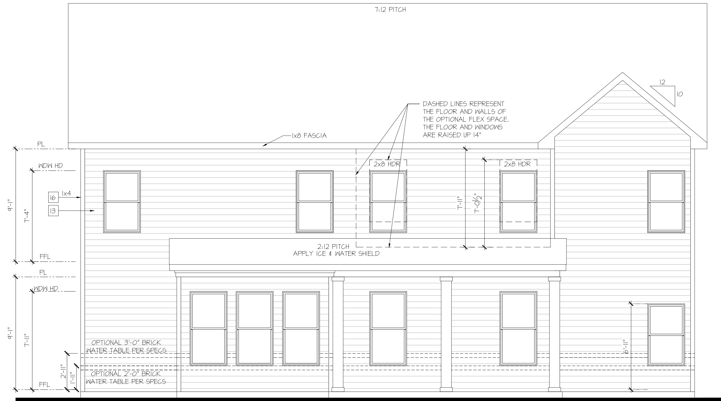
Rear Elevation w/ Opt. Covered Patio SCALE: 1/4"=1'-0" AT 22'X34" LAYOUT 1/8"=1'-0" AT 11'X11" LAYOUT
