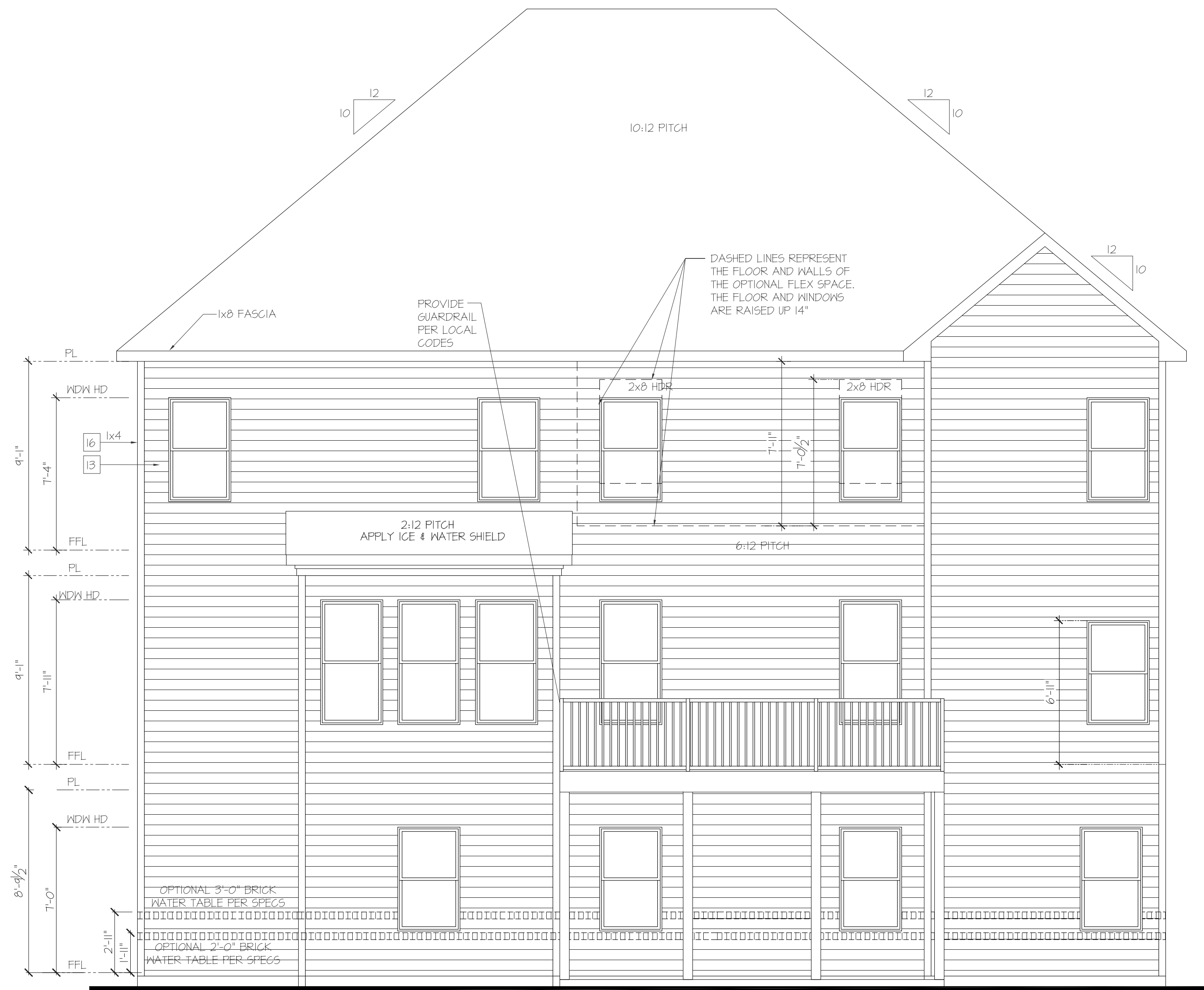
Rear Elevation Opt. Basement
