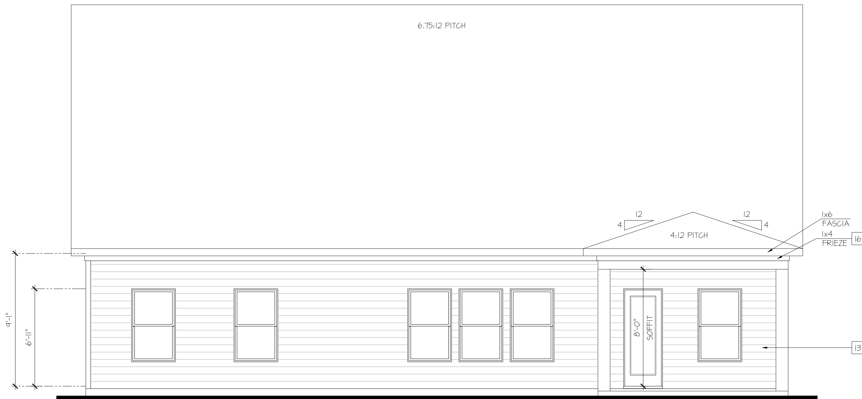
Partial Rear Elevation Opt. Covered Patio SCALE: 1/4"=1'-0" AT 22'X34" LAYOUT 1/8"=1'-0" AT 11'X11" LAYOUT
