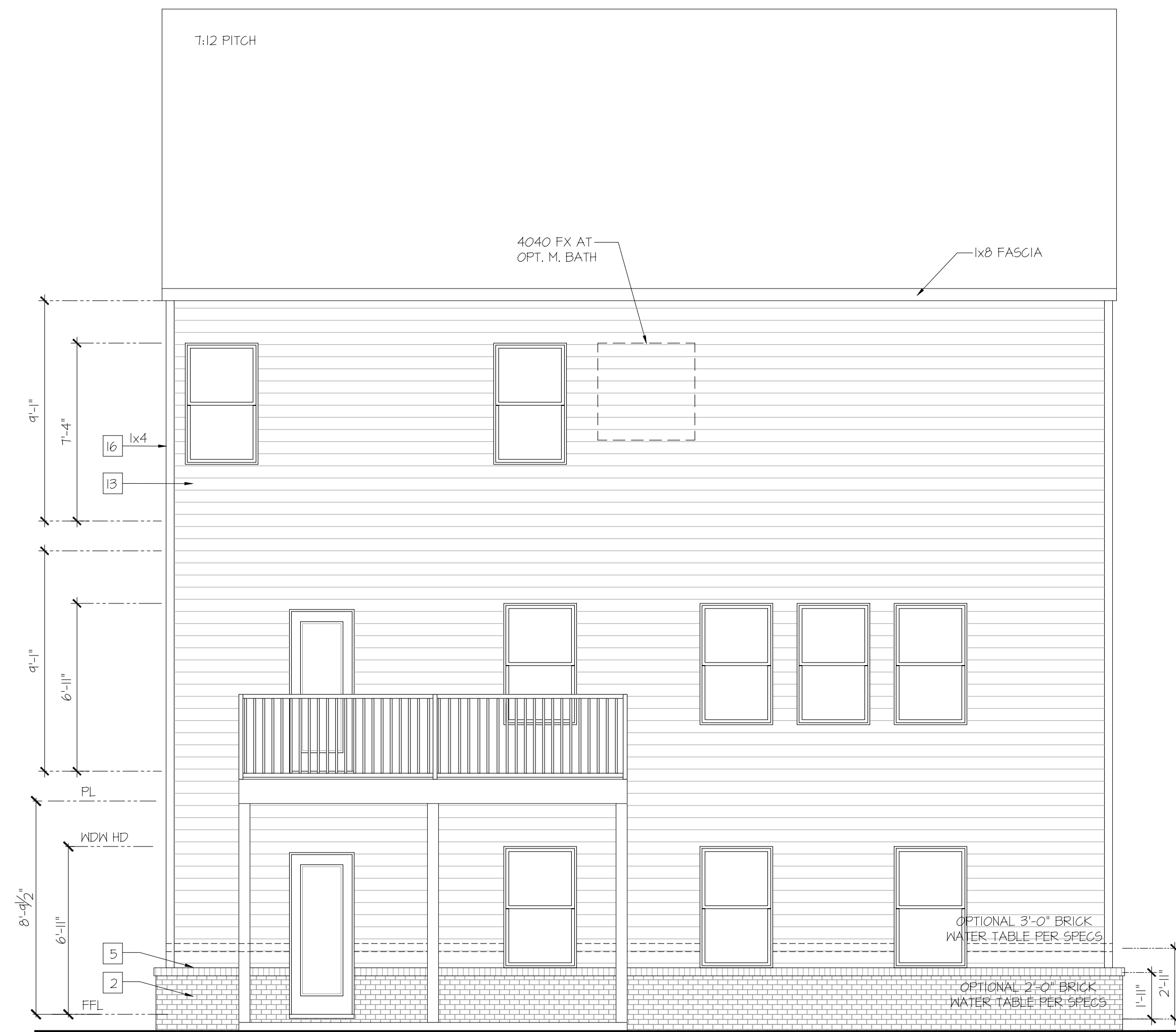
Rear Elevation Opt. Basement
