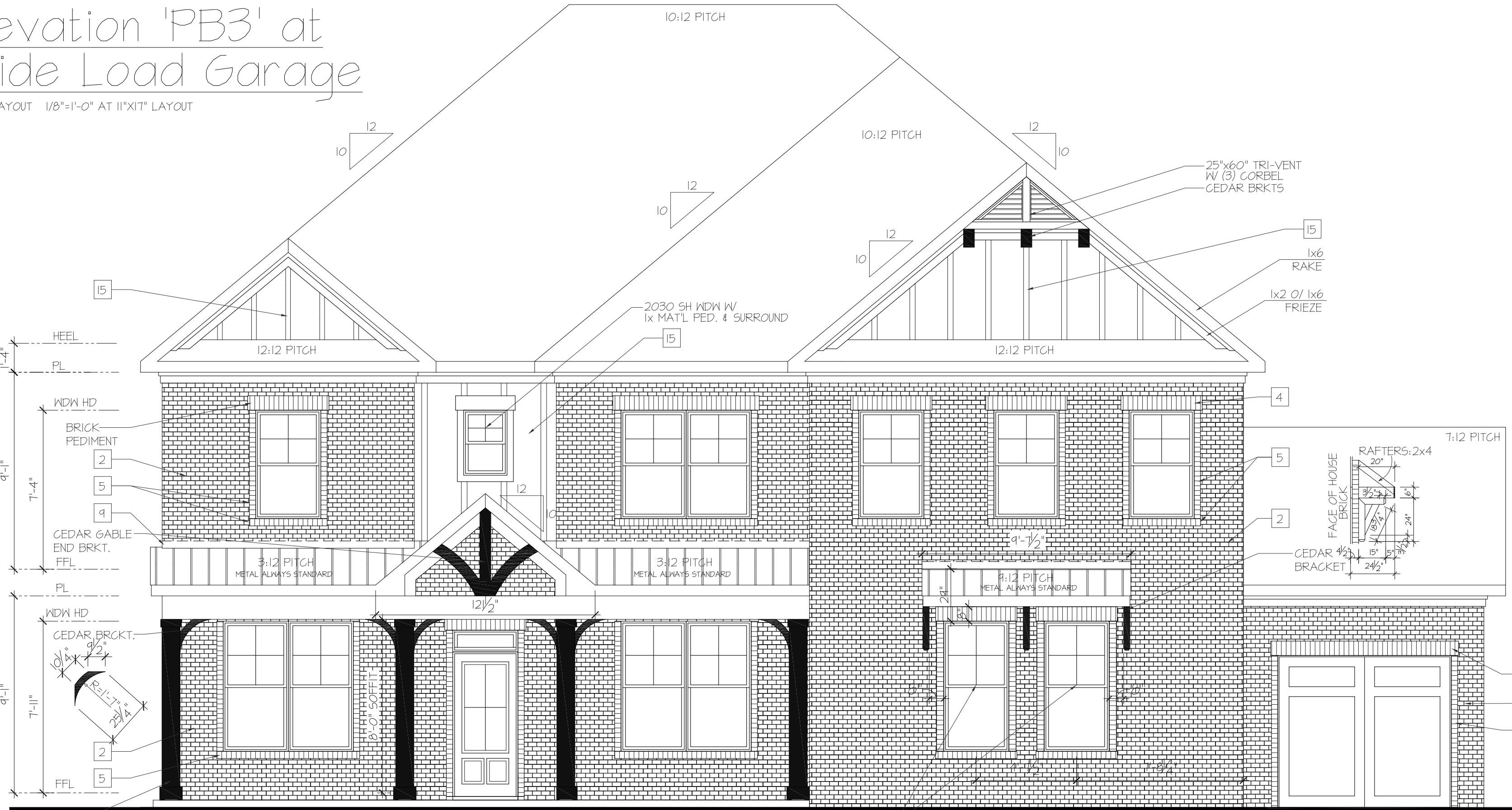
Front Elevation 'PB3' at 3-Car Side Load Garage SCALE: 1/4"=1'-0" AT 22'X34' LAYOUT 1/8"=1'-0" AT 11'X17' LAYOUT
