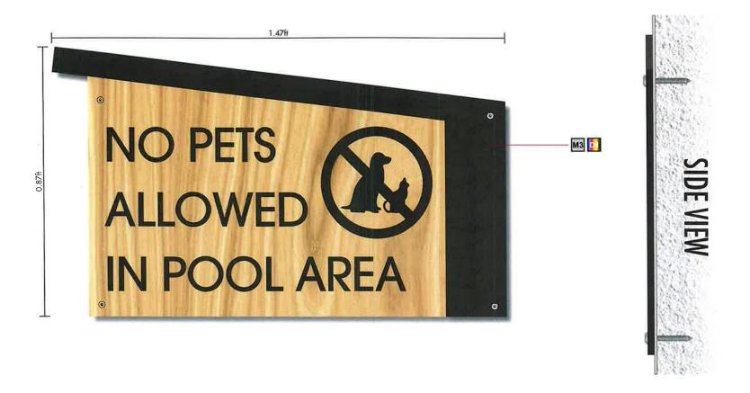
MOUNTING METHOD: MECHANICALLY FASTENED THROUGH FACE WITH 1/4"-15 BUTTON-HEAD CORROSION-RESISTANT SCREWS, MOUNTED FLUSH TO WALL
