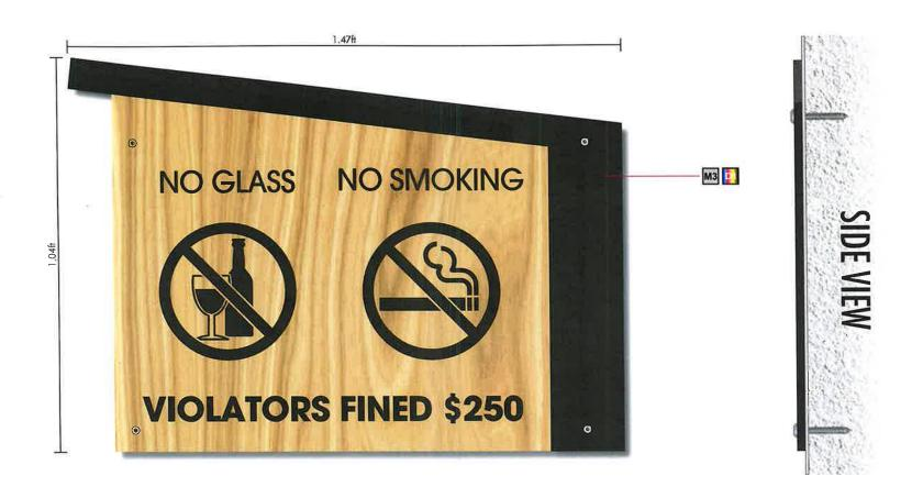
MOUNTING METHOD: MECHANICALLY FASTENED THROUGH FACE WITH 1/4"-15 BUTTON-HEAD CORROSION-RESISTANT SCREWS, MOUNTED FLUSH TO WALL
