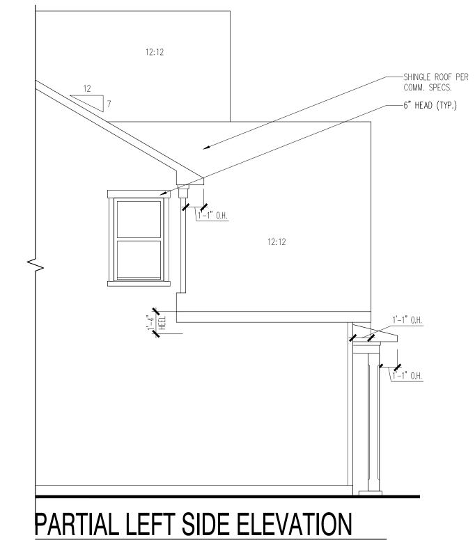
SHINGLE ROOF PER COMM. SPECS. 6" HEAD w/ 2" CAP (TYP.) 6" FRIEZE BRD w/ 2" CAP (TYP.) 20X20 FIXED 4" O.H. 4" TRIM (TYP.) 4" SILL (TYP.) 1X10 w/ DRIP CAP 1'-1" O.H. 8" HEAD W/ 2" CAP PER COMM. SPECS.
