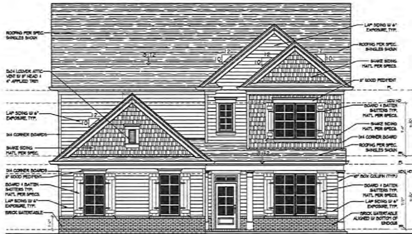
1 Front Elevation 'C' SCALE: 1/4" = 1'-0"
