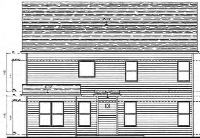
3 Rear Elevation - Standard A2.1 SCALE: 1/4" = 1'-0" 0 4' 8'
