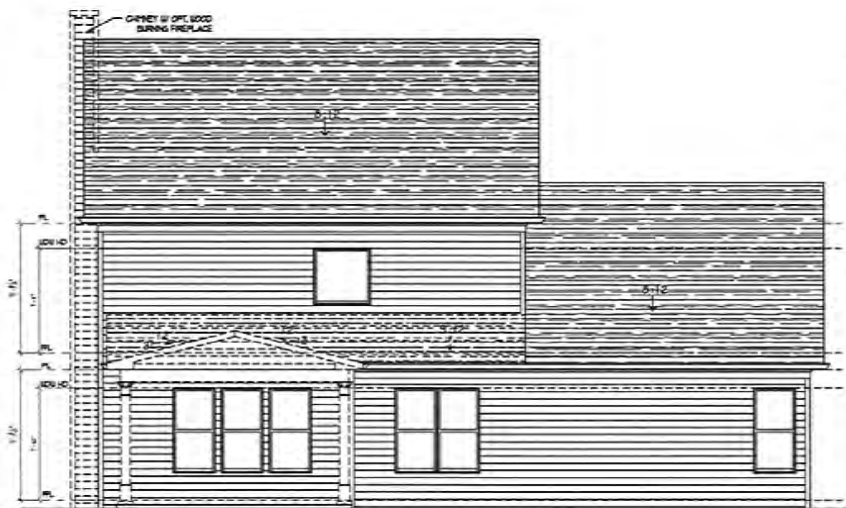
4 Rear Elevation w/ Covered Porch Opt. SCALE: 1/4" = 1'-0"
