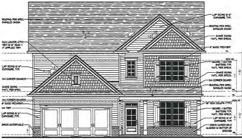
1 Front Elevation 'C' ALL SCALE: 1/4" = 1'-0" 0 4 8
