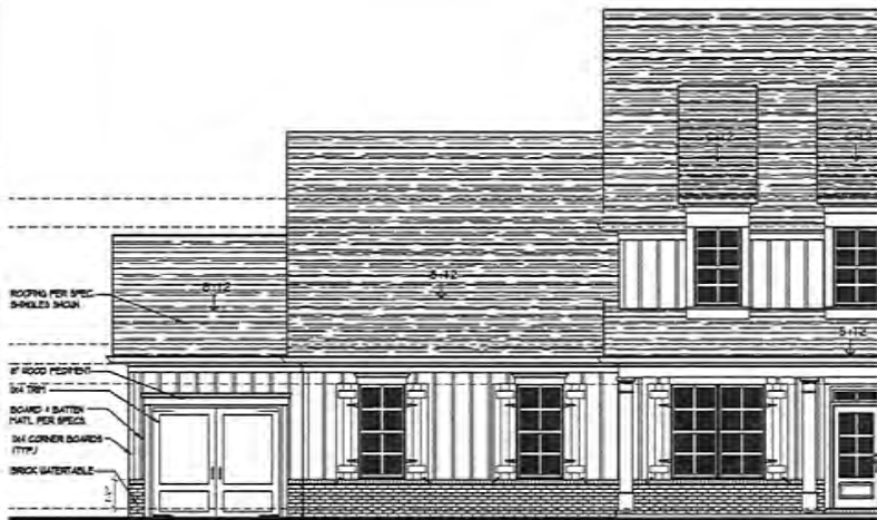
4 Front Elevation 'B' w/ 3rd Car Garage Opt.-Side Entry SCALE: 1/4" = 1'-0"
