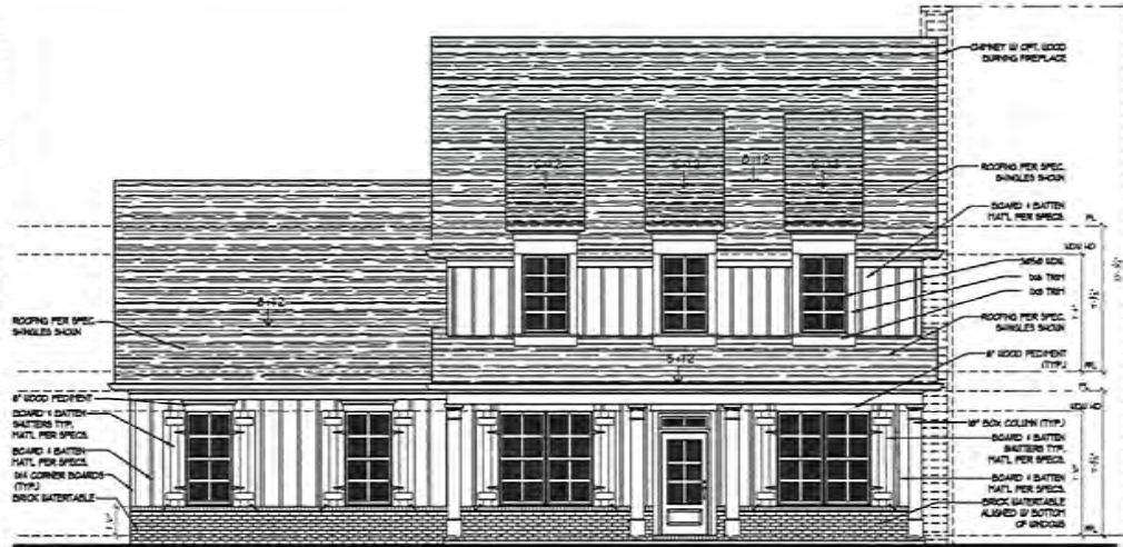
1 Front Elevation 'B' SCALE: 1/4" = 1'-0"
