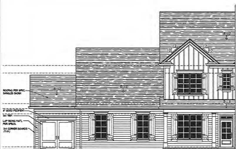
1 Front Elevation 'A' w/ 3rd Car Garage Opt. - Side Entry SCALE: 1/4" = 1'-0"
