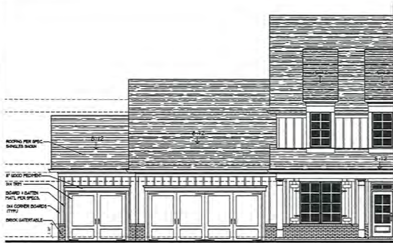
4 Front Elevation 'B' w/ 3rd Car Garage Opt.-Front entry ALL SCALE: 1/4" = 1'-0"
