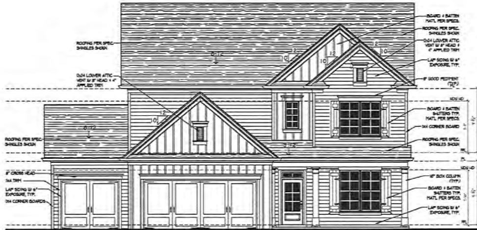
1 Front Elevation 'A' w/ 3rd Car Garage Opt.-Front entry ALL SCALE: 1/4" = 1'-0"
