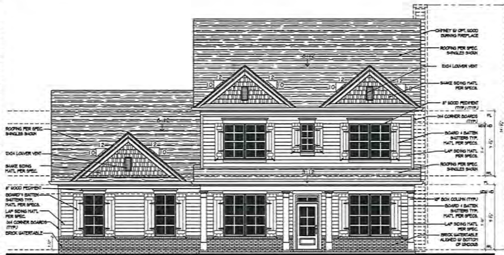
1 Front Elevation 'C' ALL SCALE: 1/4" = 1'-0"
