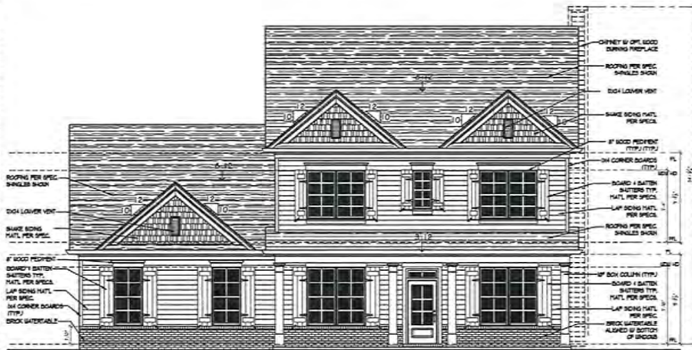
1 Front Elevation 'C' SCALE: 1/4" = 1'-0"
