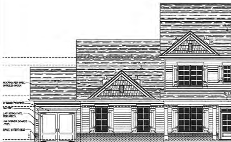
1 Front Elevation 'C' w/ 3rd Car Garage Opt.-Side Entry SCALE: 1/4" = 1'-0"
