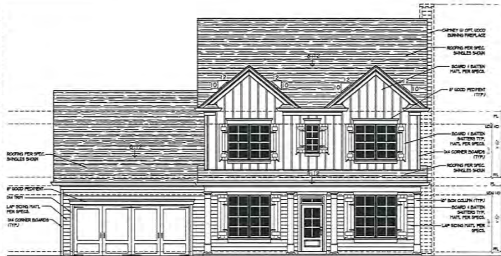
1 Front Elevation 'A' AU SCALE: 1/4" = 1'-0"
