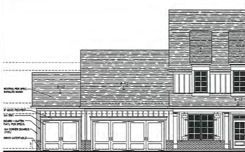
4 Front Elevation 'B' w/ 3rd Car Garage Opt.-Front entry A1.2 SCALE: 1/4" = 1'-0"
