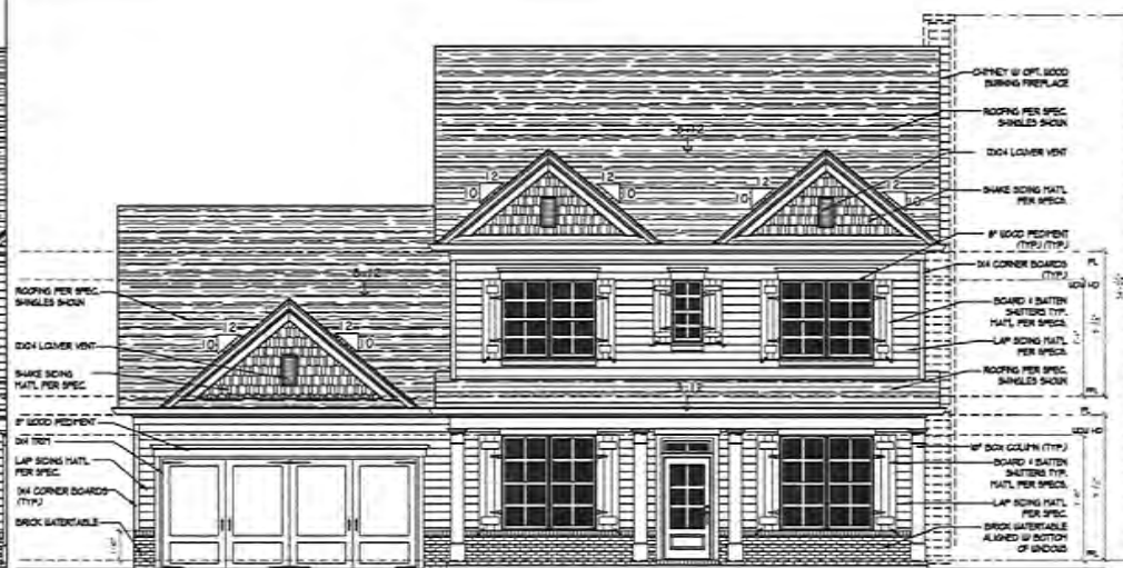
1 Front Elevation 'C' SCALE: 1/4" = 1'-0"
