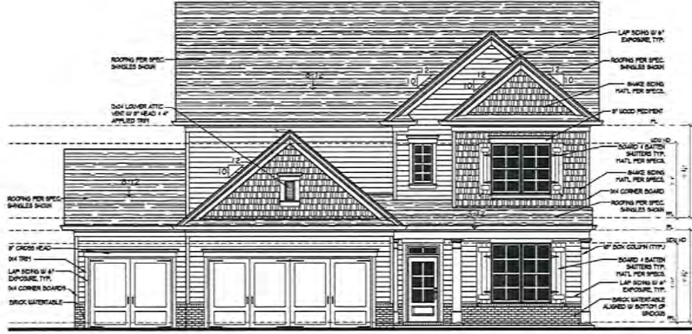
① Front Elevation 'C' w/ 3rd Car Garage Opt.-Front entry (A1.3) SCALE: 1/4" = 1'-0"
