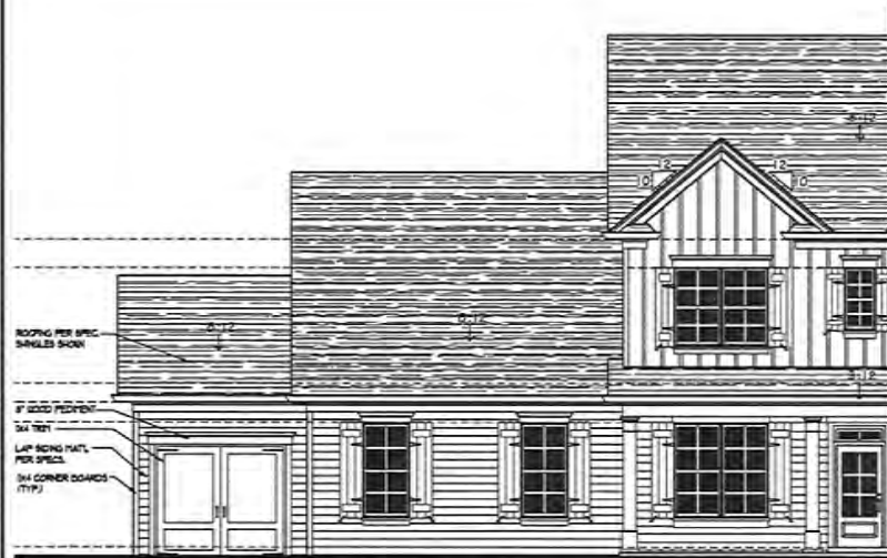
1 Front Elevation 'A' w/ 3rd Car Garage Opt. - Side Entry ALL SCALE: 1/4" = 1'-0"
