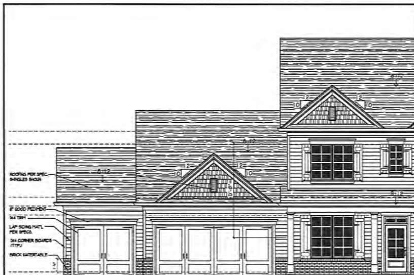
4 Front Elevation 'C' w/ 3rd Car Garage Opt.-Front entry SCALE: 1/4" = 1'-0"
