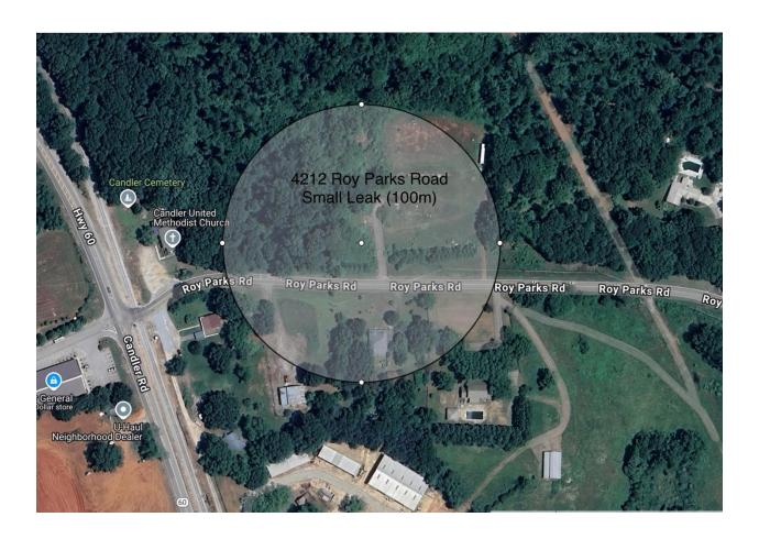
100m (328ft) Small Leak Initial Isolation Distance 55 gallons, 200lbs, or 200 cubic feet or less
