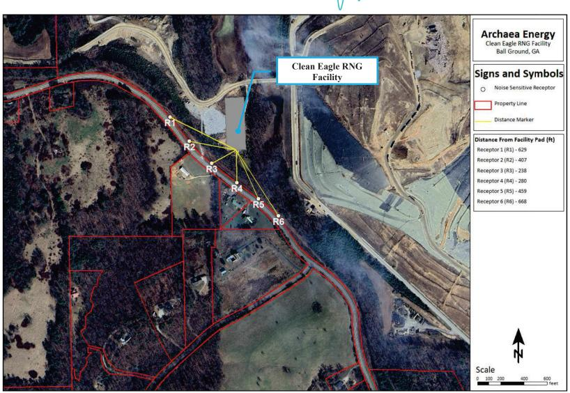
Figure 3 Site and Noise Sensitive Receptor Location
