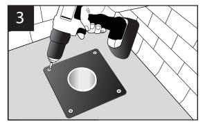
Secure stabilizer to sub floor with screws or nails.
