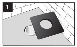
Mark and cut pipe so that top of pipe is slightly above floor level. Use the base of the stabilizer to measure proper pipe height.
