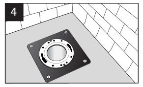
Install closet flange on top of Closet Flange Stabilizer.
