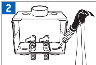
2 Hit screwdriver until it penetrates under test cap.
