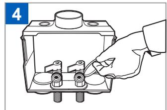
4 Reach in with hand or pliers and remove test cap.
