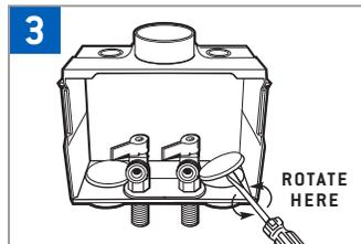
3 Rotate screwdriver lifting up test cap.
