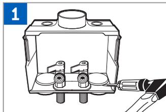
1 Position flathead screwdriver at intersection of bottom wall and raised test cap.
