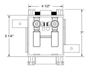
Specifications: Furnish and install fire-rated MultiBox Single Washing Machine Outlet Box. Unit shall be Water-Tite product code checked below, as manufactured by IPS Corporation.
