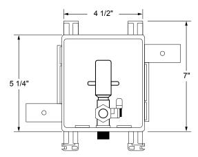
**Specifications:** Furnish and install fire-rated MultiBox Ice Maker Outlet Box. Unit shall be Water-Tite product code checked below, as manufactured by IPS Corporation.
