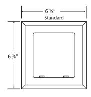
**Specifications:** Furnish and install MultiBox Washing Machine Outlet Box and Auxiliary Drain Box System. Boxes may be inter-connected or installed separately. Valve box includes DWV drain to capture hose leaks, while the drain box contains 2" drain with inte-grated knock-out for DWV testing. Unit shall be Water-Tite product code checked below, as manufactured by IPS Corporation.
