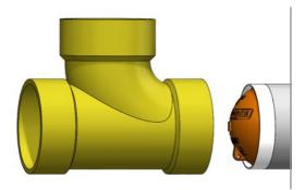
5. Locate sanitary tee and prepare to solvent weld SCO Test Plug/pipe assembly together.
