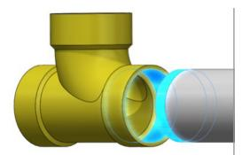
7. It is recommended to only apply primer to the ID of the sanitary tee. Solvent can be applied but sparingly, too much will cause the cap to permanently lodge into assembly.
