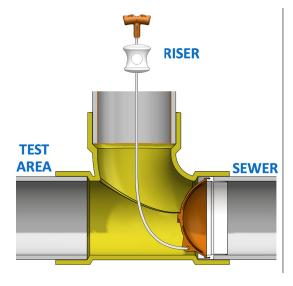
10. After test, unravel remaining rope to remove t-handle from styrofoam float, then remove slack and pull to remove cap from sanitary tee assembly.
