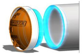
3. Apply primer and solvent to the flange of the SCO and to the ID and top of the end of the pipe. \*It is important for no primer or solvent to make contact with the region where the cap meets the body of the SCO plug. This can cause leaking when pressure testing.
