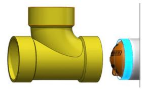
6. Liberally apply primer and solvent to OD of body of the SCO Test Plug and pipe. Application of primer and solvent should be to socket depth.\*Pull tab must be in downward position. See arrows on cap. It is important for no primer or solvent to make contact with the region where the cap meets the body of the SCO plug. This can effect the seal and cause leaking when pressure testing.
