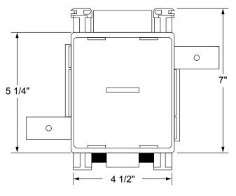
**Specifications:** Furnish and install fire-rated MultiBox with Redi-Vent Kit. Unit shall be Water-Tite product code checked below, as manufactured by IPS Corporation.
