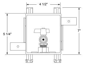
**Specifications:** Furnish and install fire-rated MultiBox Gas Outlet Box. Unit shall be Water-Tite product code checked below, as manufactured by IPS Corporation.
