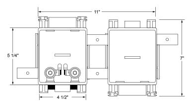
Specifications: Furnish and install fire-rated MultiBox Two-Box Washing Machine Outlet Box System. Boxes may be inter-connected or installed separately. Valve box includes DWV drain to capture hose leaks, while the drain box contains 2" drain with integrated knock-out for DWV testing. Unit shall be Water-Tite product code checked below, as manufactured by IPS Corporation.
