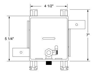
**Specifications:** Furnish and install single MultiBox Washing Machine Outlet Box and MultiBox Ice Maker Outlet Box. Units shall be Water-Tite product codes checked below, as manufactured by IPS Corporation.
