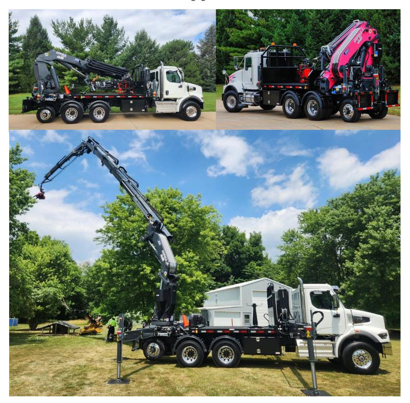
The Copma 650.6J6 has 6 main extensions and 6 jib extensions allowing for a 1,590 lbs. at 94' 4" horizontal reach and 1,930 lbs. at 107' vertical reach.
