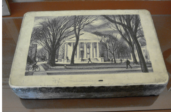
Figure 2.15 | Stone used for lithography print
