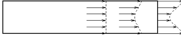
Figure 2.2: Internal force behavior in bars
