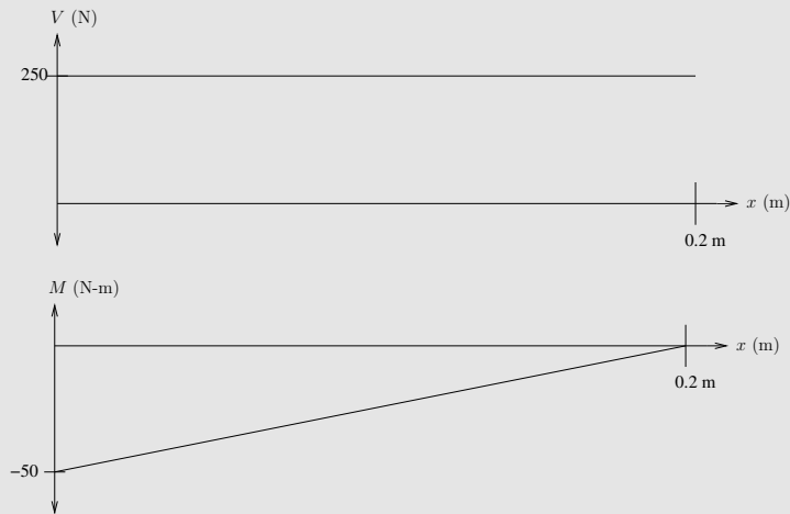
Figure 5.31: Shear and moment diagrams for Example 5.6
