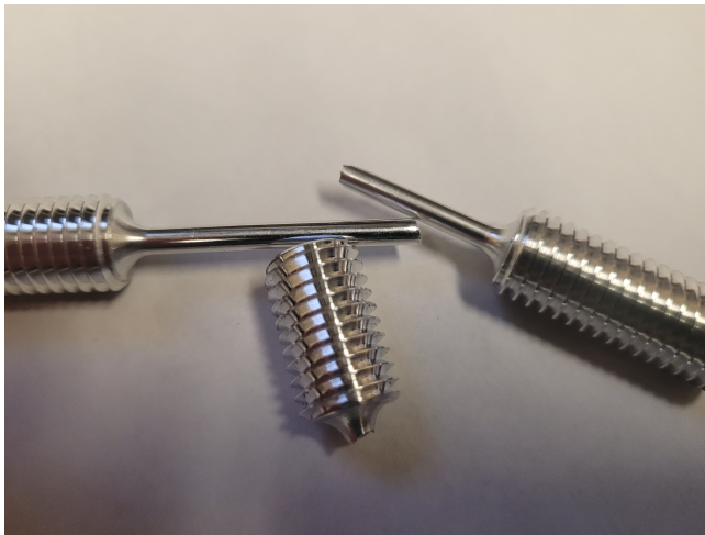
Figure 1.32: Brittle failure of an aluminum sample
