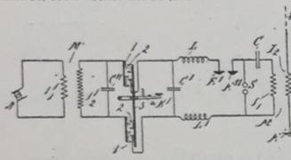
1. A space telegraph transmitting system comprising a sonorous circuit, a power circuit including the primary of a transformer, an intermediate circuit connected with said sonorous circuit and including the secondary of said transformer, and means associated with said intermediate circuit for increasing the power factor of said power circuit.
