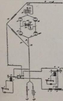
1. The combination with a circuit, and means for impressing thereon currents of varying strength and of reversed polarity, of a neutral relay and a series of relays between the said relay and said circuit and so disposed as to commutate said currents, whereby all of said currents will pass through the relay in the same direction, substantially as and for the purposes set forth.
