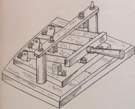
It would be well to measure the distance between the outside poles of the switch before boring holes in crosspiece as when the switch is thrown up these poles should fit in the clips on the crosspiece.
