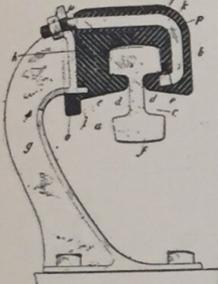
1. A two-part third-rail insulator, each part having a flange to support the rail, and one part overlapping the other part so as to cover the joint between the two parts.
