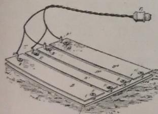
1. An electric trap comprising an insulated base and a series of conducting plates separated from each other and supported on said base but insulated therefrom, and positive and negative wires adapted to be connected with a source of electrical energy and with alternate plates.
