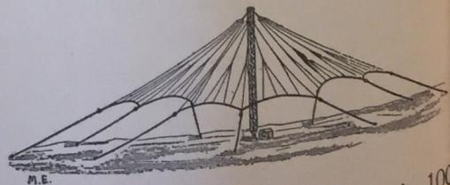
total height of the center mast is 100 meters, from which the aerial wires radiate in all directions.
