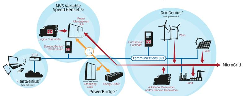
**PowerBridge™** is our energy buffer and stabilizing load system which manages overproduction of renewable generation and allows engine off and stabilization of third party fixed speed generators.
