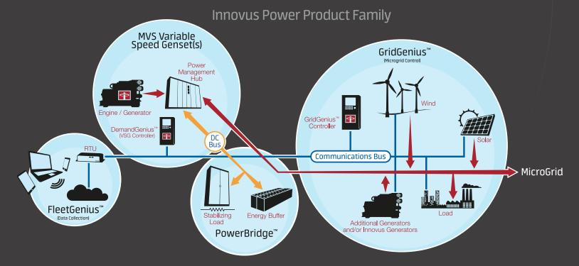
**PowerBridge™** is our energy buffer and stabilizing load system which manages overproduction of renewable generation and allows engine off and stabilization of third party fixed speed generators.
