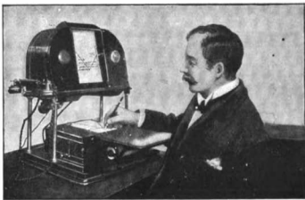
THE TELAUTOGRAPH WILL TRANSMIT MESSAGES IN THE ACTUAL HANDWRITING OF THE SENDER.
