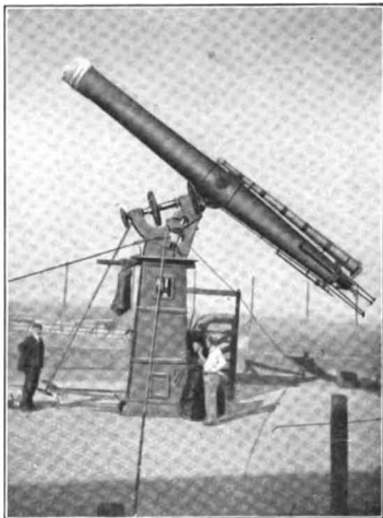
THE EIGHTEEN-INCH REFRACTING TELESCOPE USED BY PROFESSOR TODD IN OBSERVING AND PHOTOGRAPHING MARS
