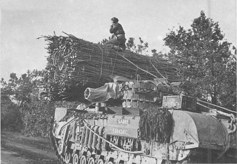
Special tank "Petard" with fascines (loaded at front) moves up to battle. ( British official photo )
