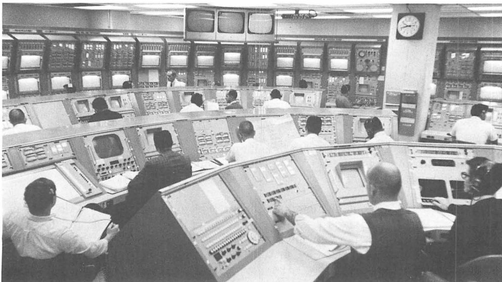
An Apollo spacecraft is checked out from this room at KSC, using the automated Acceptance Checkout Equipment developed for the program.
