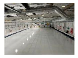
The ice pad floor has been covered in a new vinyl surface - this has reduced the time spent painting the floor - and will now mean that the painstaking task of removing paint at the end of the season is no longer required.
