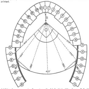
Additional measurements: Concrete wall—14 ft. high; Wire fence—7 ft. high. 5
