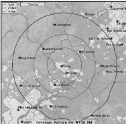
Coverage map of 91.3 WTSR, located on the campus of The College of New Jersey in Ewing (courtesy Radio-Locator.com)
